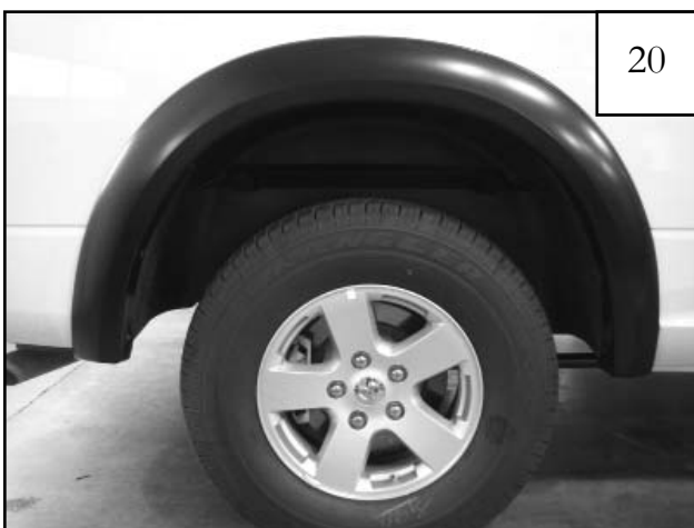
Completed rear flare installation.
