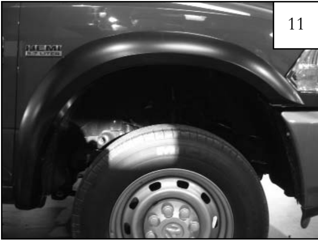
Completed front flare installation.
