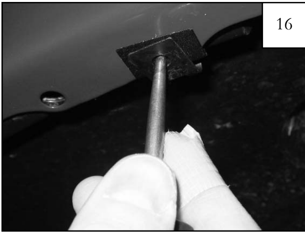
Using an awl or similar pointed tool, poke a hole through 1"x1.5" Black Tab using the #10 U-Clip hole as a guide.
